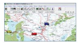
Internav® CHF is an Automatic Vehicle Location and Tracking system that uses Navstar Global Positioning System (GPS) and CODAN™ HF Transceivers to exchange position data between mobile stations and a central control station. The MS Windows™ based tracking software, located at the control station, acquires position data from selected mobile stations and then plots their positions on a computer based map.
